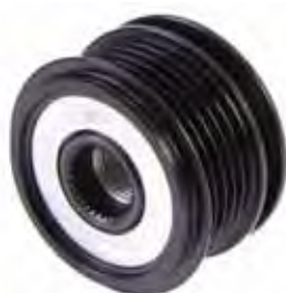
OAP005 BORE 33 TOOTH SPLINE TYPE 5PK OD 57mm V 18.47mm ID 17mm W 41mm THREAD M16
