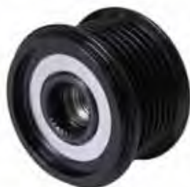
OAP013 BORE 33 TOOTH SPLINE TYPE 7PK OD 52.6mm V 8.8mm ID 17mm W 39.4mm THREAD M14
