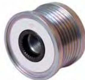
OAP0012 BORE 33 TOOTH SPLINE TYPE 6PK OD 50mm V 13.8mm ID 17mm W 40mm THREAD M17
