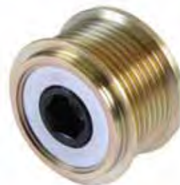
OAP008 BORE 17MM HEX TYPE 7PK OD 58mm V 11.24mm ID 15mm W 42.5mm THREAD M14
