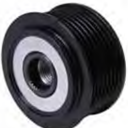
OAP0015 BORE 33 TOOTH SPLINE TYPE 7PK OD 65mm V 10.2mm ID 17mm W 40.8mm THREAD M17
