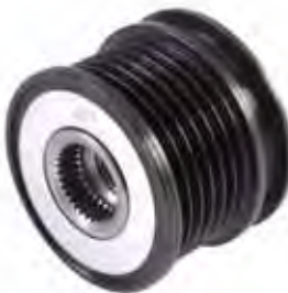
OAP007 BORE 33 TOOTH SPLINE TYPE 6PK OD 49.8mm V 14.69mm ID 17mm W 39mm THREAD M16
