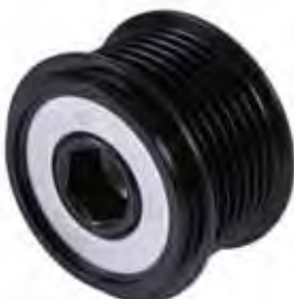
OAP0010 BORE 17MM HEX TYPE 7PK OD 55.3mm V 9mm ID 17mm W 40.6mm THREAD M14
