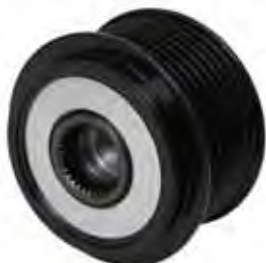
OAP0014 BORE 33 TOOTH SPLINE TYPE 7PK OD 60mm V 8.65mm ID 17mm W 41.5mm THREAD M16
